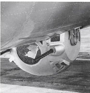
The ball (belly) turret of a B-17. Howard once said that during combat it seemed like there was just a small piece of glass between him and the ground.
